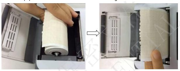
Loading/Replacing Process of Rolled Thermal Paper
