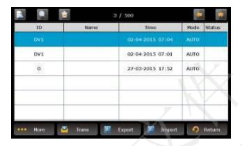
The File Manager allows records to be stored, deleted, printed and transmitted. When there is no space for more records to be stored in the File Manager, the message *MemFull* will be displayed.
