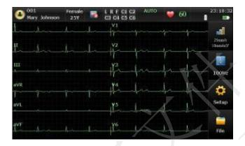
On the main screen, the following information is displayed: patient information, system hints, heart rate, waveforms, current time, battery capacity, WIFI signal (optional), and functional keys.
